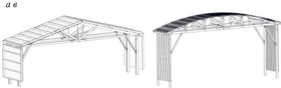
Fig. 9. The frame panel section unit with the collar beam in the form of the truss unit *a* and the roof unit *б*
